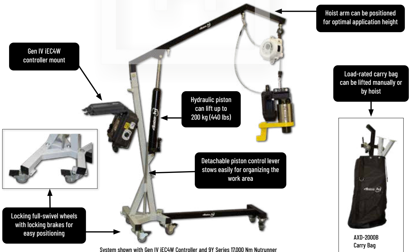
System shown with Gen IV iEC4W Controller and 9Y Series 17,000 Nm Nutrunner Controller and tool sold separately
